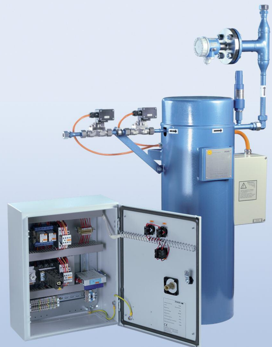
Ammoniac vaporizer with trap for liquefied gas type ETA Indirect electric heating system 5-30 kg/h
